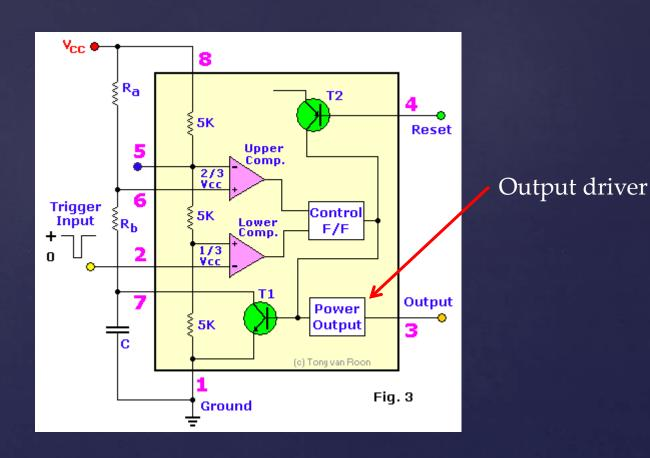
By adding just three external components (2 resistors and a capacitor) we can create many different circuits:
