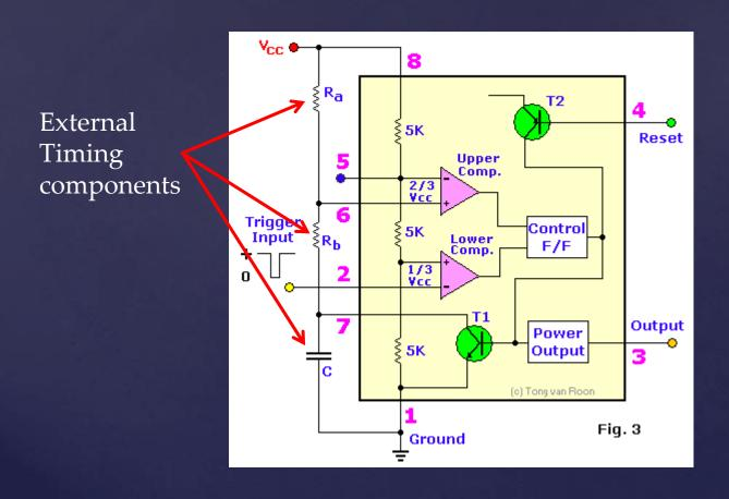
An *oscillator* is a device that can produce a series of pules (think 1's and 0's) at a specific *frequency* or *duty cycle*:
