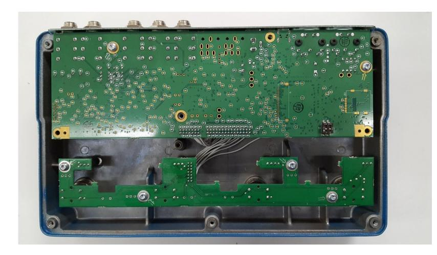
• Opening up the bottom of the enclosure reveals some very well engineered design approaches. You will notice that there are multiple PCBs. Ribbon cables connect the different boards together.
