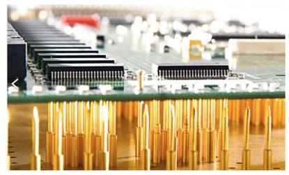
Bed of nails with and without a PCB mounted. The gold pins are called "pogos" and are spring-loaded contacts to make a non-soldered electrical connection to the board. • Electrical connections are made with ribbon cables that allow rapid assembly without extra soldering.
