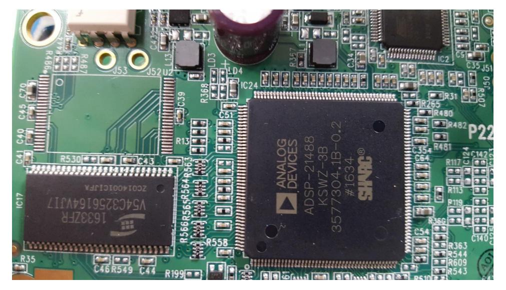
• Surface mount technology (SMT) is used extensively in this design. The IC on the right is a Digital Signal Processor (DSP), often used in Cell Phones and other audio equipment. The I.C. on the left is most likely a memory chip for storing the processed analog signals.
