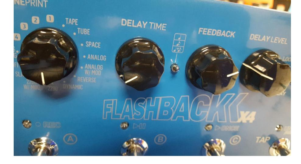
• This is a top view of the knobs and switches. Each of these are connected with the mini-PCBs on the bottom.
