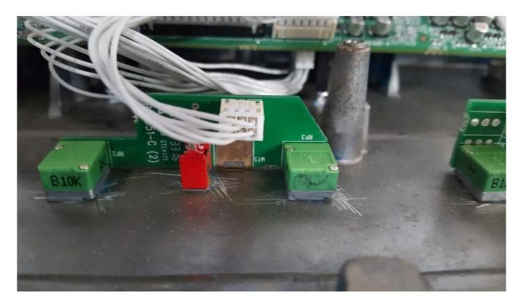
• Close-up view of a PCB that has a square potentiometer and red toggle switch. This takes care of the right angle mounting problem if you tried to mount these parts on the main board.
