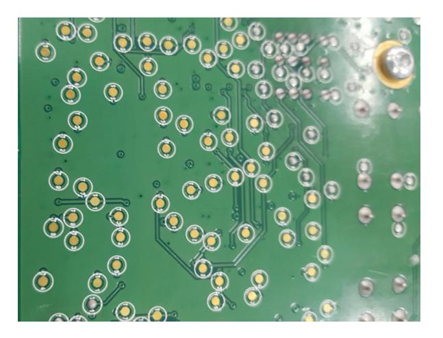
• At first you may not realize what all of these gold pads are. These are actually test points for performing electrical tests (using a bed of nails) and downloading code to the processor prior to assembly! Better to test before putting the whole assembly together...
