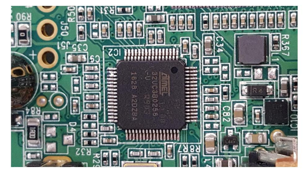
• Close up view of the microprocessor – this is similar to the same part used in Arduinos!!
