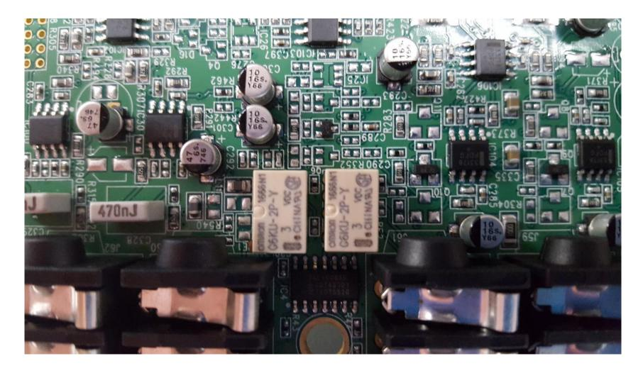
• Although by far the majority of the parts are SMT, there are a few that are through-hole, like these little relays. For larger components, or ones that require more current, you still often need to use through-hole components.
