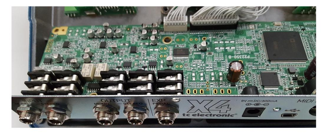
• This view shows how right angle audio connectors are used to connect to the back panel. This allows fast assembly with a number of connectors. Notice the mini-USB connector on the right for downloading different sounds.
