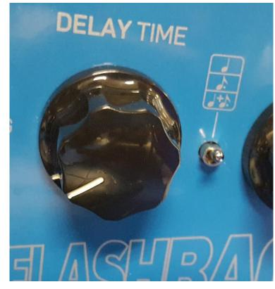
• Top view of the POT with a knob and the toggle switch
