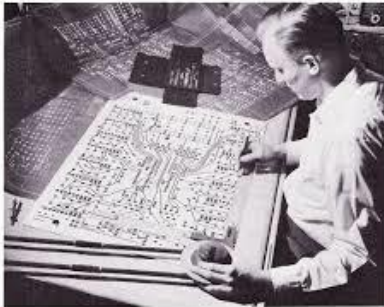
no. 19.34. Drawing a printed circuit. The drawing is carefully planned and executed for photographic reproduction on the circuit board.
